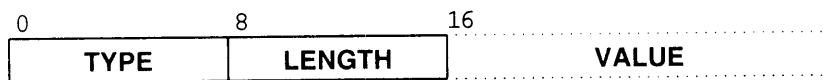
Figure 33.7 Encoding of an individual option in an IPv6 option extension header. Each option consists of a one-octet type and a one-octet length followed by zero or more octets of data for the option.
